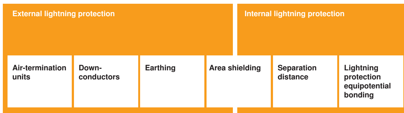
External and internal lightning protection systems
