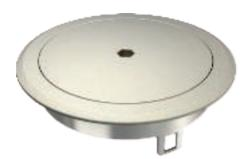
Blanking lid with Allen slot for GES R2 floor socket for direct installation in the MT R2 installation socket. The lid exit can be used as a cable outlet. When closed, the floor socket fulfils the requirement of EN 50085-2-2 for wet-cleaned floors.
