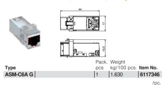
Connection module Cat. 6A (ISO) shielded, with a RJ45 slot. Including an EMC screen hood, a dust cover, a cable tie, a Keystone fastening frame and mounting instructions. Suitable for installation in the data technology supports of type DTG-2C and DTS-2C, support plate of type MTM 2C and MTM 3C, mounting plate of type MPR2 2C, mounting supports of type MTGE2 2C, MTGE2 15 2C and MTGE2 F 2C.
