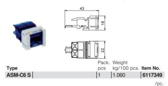
Connection module Cat. 6 unshielded, with a RJ45 slot. Including a dust cover, a cable tie, a snap-in fastening frame and mounting instructions. Suitable for installation in support plates, type MTM 2C and MTM 3C, mounting plate type MPR2 2C, mounting support type MTGE2 2C, MTGE2 15 2C and MTGE2 F 2C.
