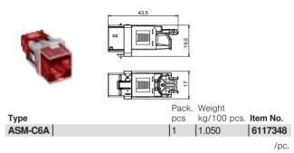
Connection module Cat. 6A (ISO) unshielded, with a RJ45 slot. Including a dust cover, a cable tie, a Keystone fastening frame and mounting instructions. Suitable for installation in the data technology supports of type DTG-2C and DTS-2C, support plate of type MTM 2C and MTM 3C, mounting plate of type MPR2 2C, mounting supports of type MTGE2 2C, MTGE2 15 2C and MTGE2 F 2C.
