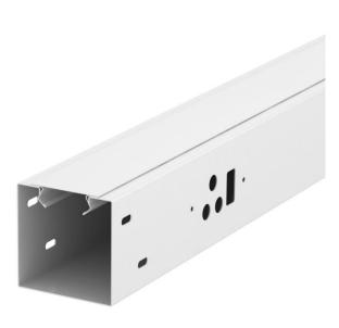
Supermarket trunking system for suspended mounting. The system is used for cable routing and device installation. Trunking length with perforations for device installation. The prepunched trunking contains the following perforations for every 3 m in length: 6x Crabtree 16A SSO, 4x insulator, 4x 32A and 5x Pin Panel socket.
