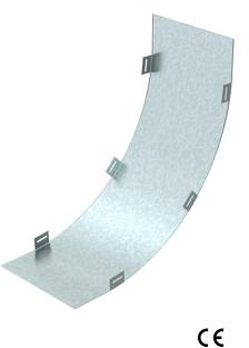
Unperforated cover for 90° vertical bend, rising, of types PT38 and PT76. Accessory radius = 450 mm. Accessory radius for 650 mm and 1000 mm available on request.
