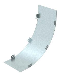
Unperforated cover for 90° vertical bend, rising, of types PT38 and PT76. Accessory radius = 450 mm. Accessory radius for 650 mm and 1000 mm available on request.
