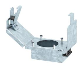
Device support of nominal size 2 for the installation of a CEE plug connection 16 A or 32 A for installation in service outlets and cassettes of nominal size 2, 4, 6 and R7. Device support with protective housing and strain relief. Required minimum installation depth: 190 mm when using a straight connector and 160 mm when an angled connector is used.
